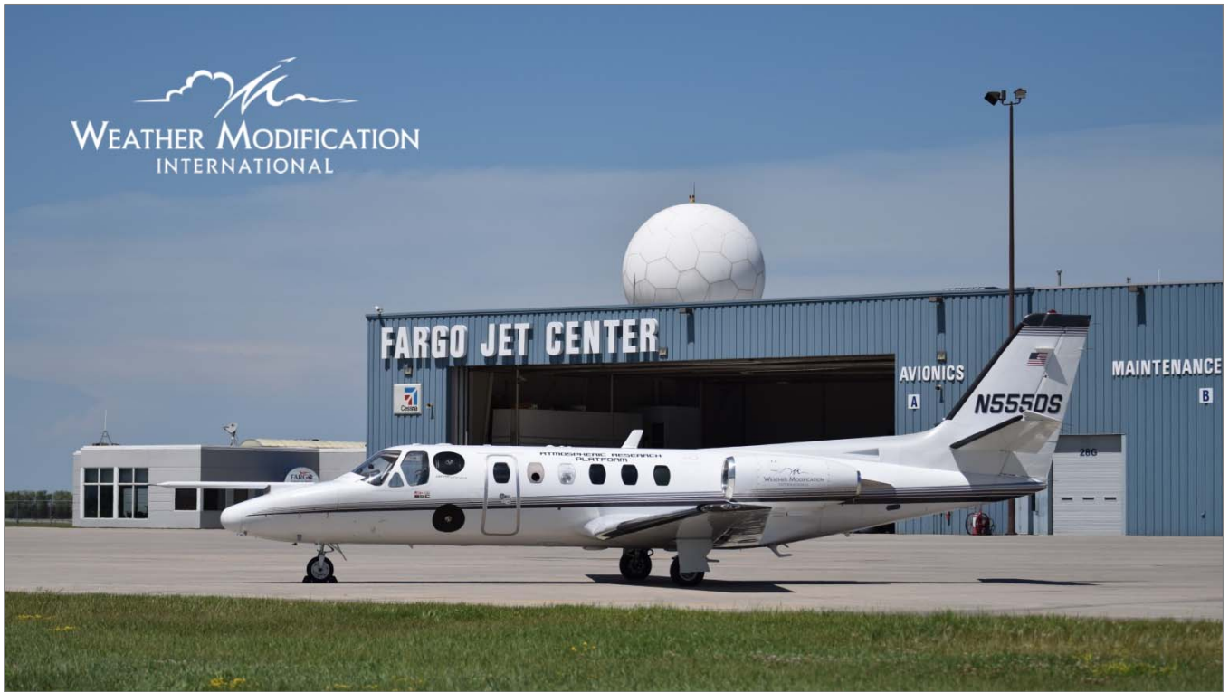
WMI Citation II, N555DS equipped with NASA Field Mill sensors (black round circles) prior to a deployment in cooperation with the Research Application Laboratory and Aerospace Corporation in August 2017.
